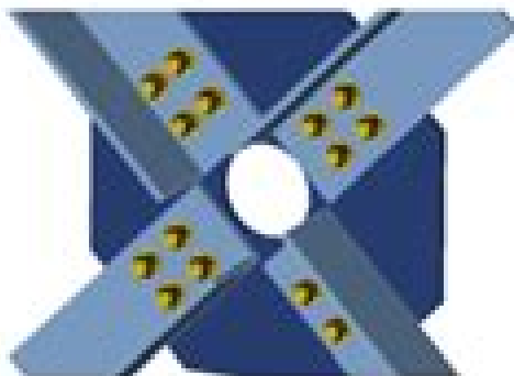
Bolted gusset plate truss connections
