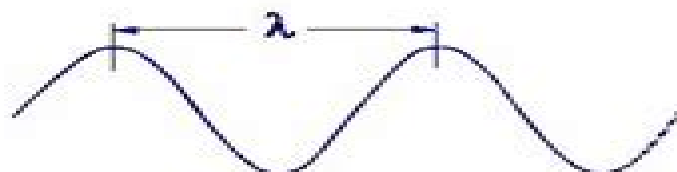
Figure 1 The wavelength \lambda of electromagnetic radiation
