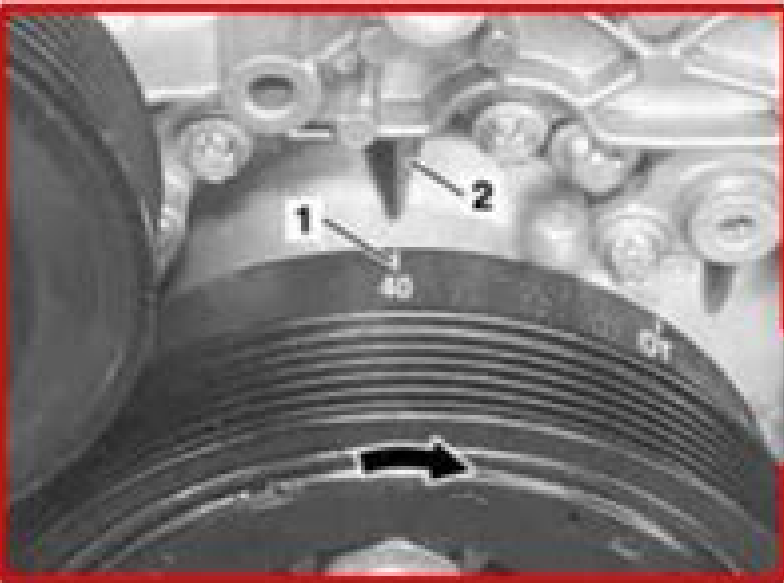
Mercedes-Benz M272 Engine Timing Marks
