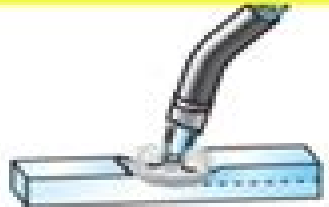
Gas-metal arc welding
