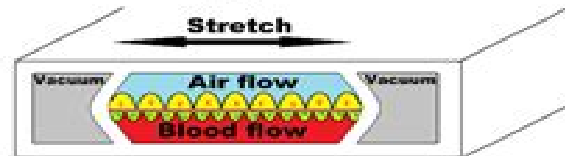
Lung on chip device to mimic breathing human lung
