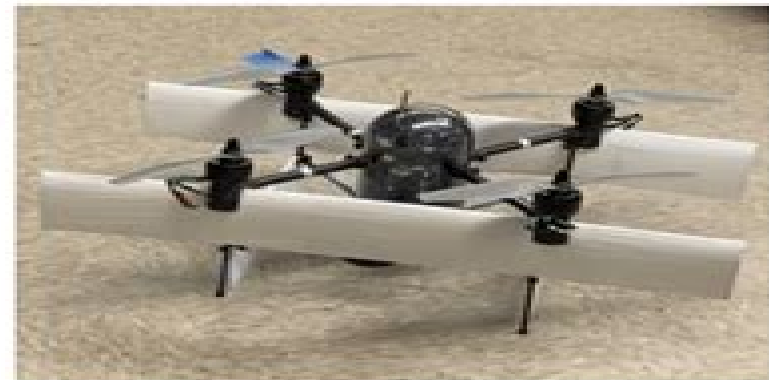
Figure 1: The 3 lb. Common Research Configuration (CRC-3) (Ref. 6)
