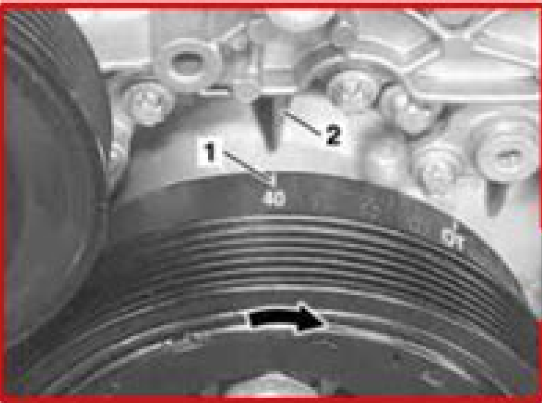
Mercedes-Benz M272 Engine Timing Marks
