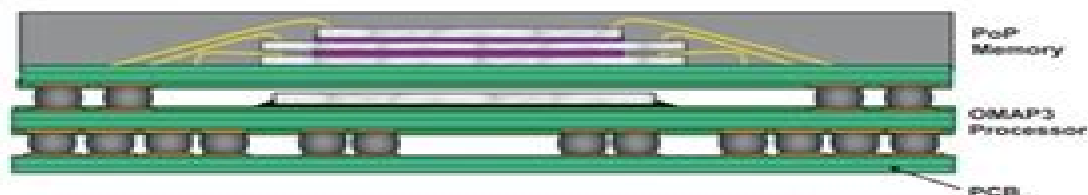
Figure 1. OMAP35x Processor (bottom device) and PoP Memory (top device) Stack Up on PCB
