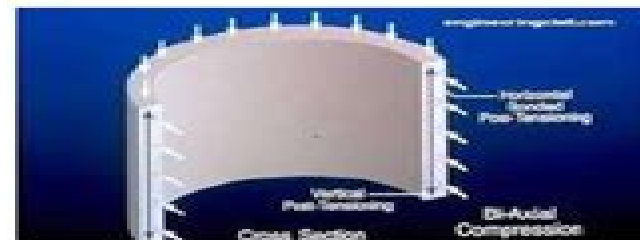
Fig. 1: Cross Section of Prestressed concrete tank
