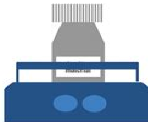
record time and place bottles on a rotary shaker incubate at 150 rpm for the chosen length of time
