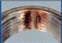
① Phenomenon: Flaking on Grooves, Spalls, Grooves, Ring Ribs ② Cause: Incorrect Handling during Assembly
