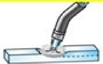
Gas-metal arc welding
