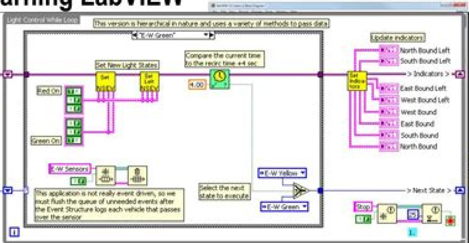
A version of the Stop Light VI that uses an Event Structure. Data is passed from the Event Structure via Notifiers and Queues.
