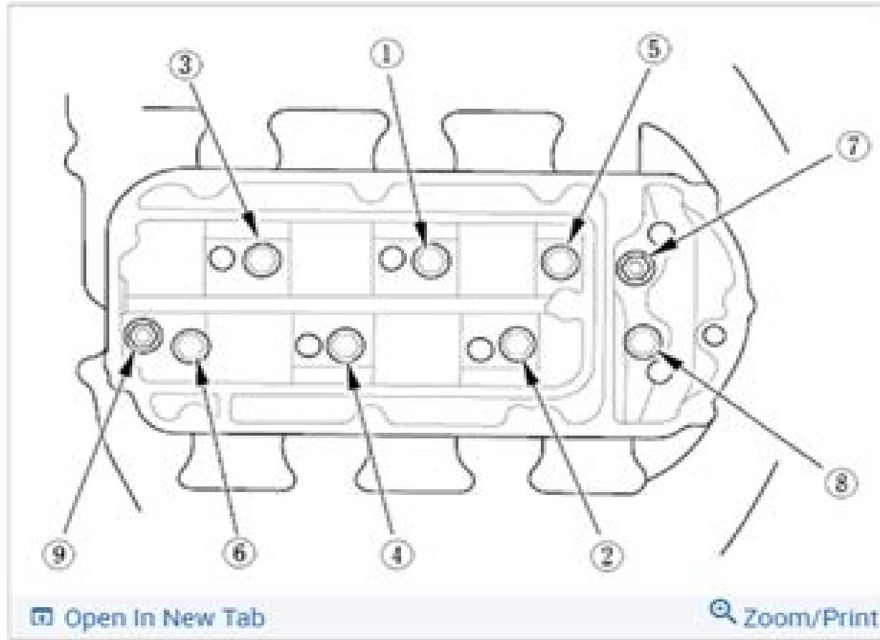
Install the [upper cover](#) (A). Tighten the bolts and nuts sequentially in three steps. Always use a new gasket.
